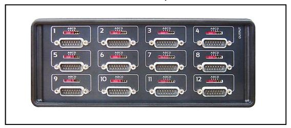
Connect the AVI units to any socket of the sensor rear panel.
